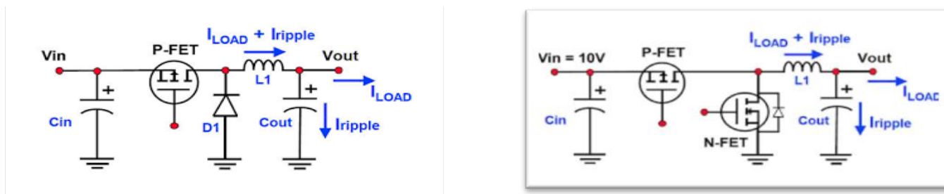
Figure 1: basic & synchronous buck dc- dc converter circuit.
